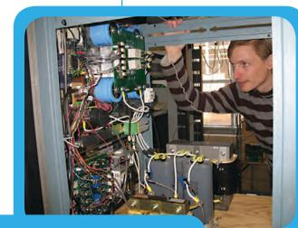
Almost all university electric power engineering programs have power electronics courses. Here an electrical engineering masters student is using a prototype to test his design of a power electronics system for integrating energy storage devices into a microgrid. New engineering skills are needed for work on the future power grid.
